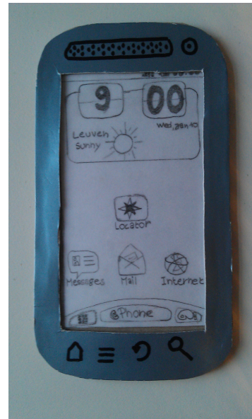
Figure 1. The prototype of the smartphone is made out of strong cardboard paper.
